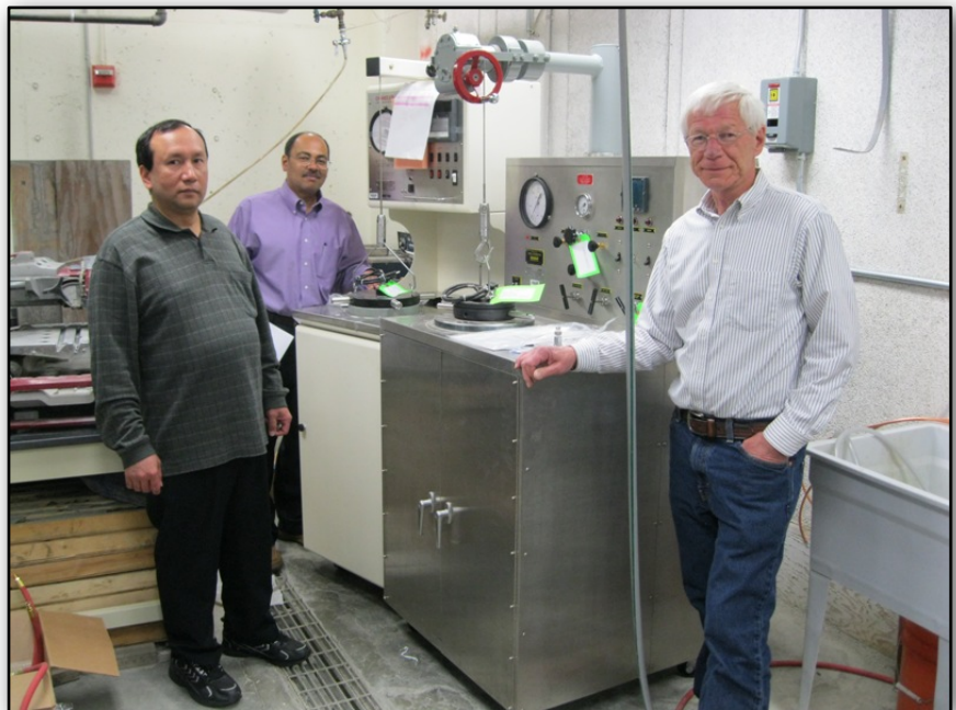
Pictured are left Dr. Santanu Khataniar, center Dr. Abhijit Dandekar and right George Trabits. Equipment is Chandler 8340 Consistometer and Chandler 1910 Curing Chamber.
